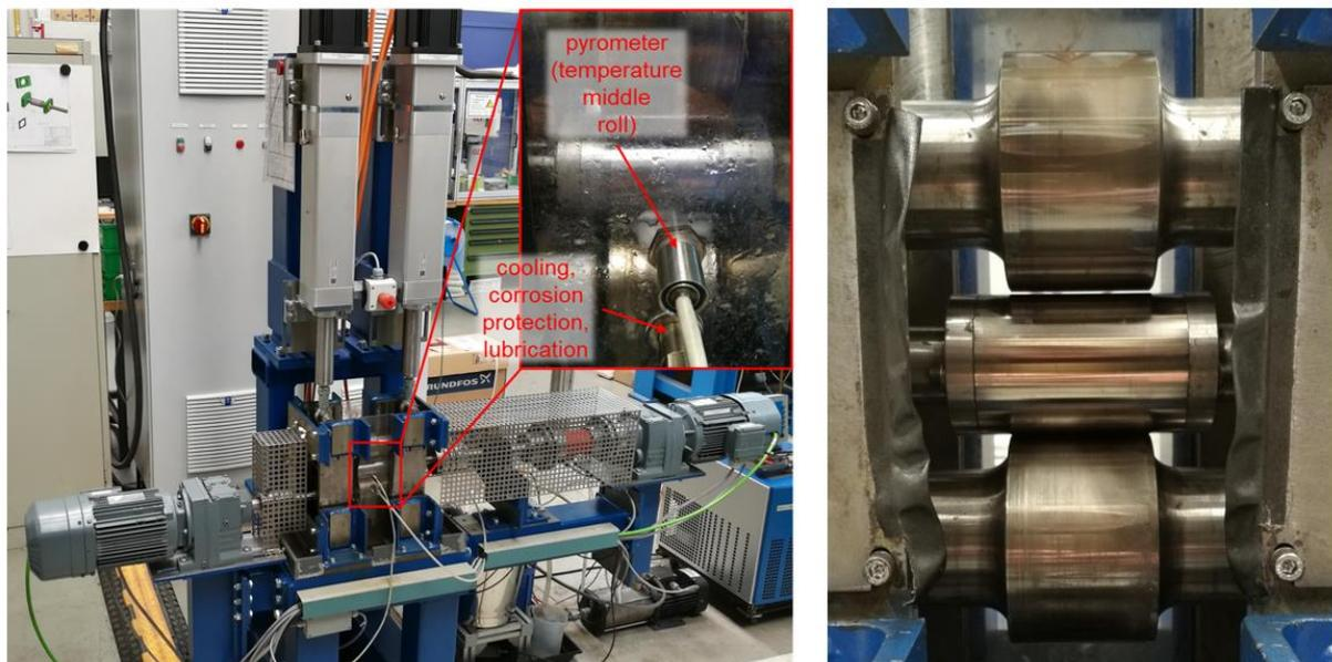
Figure 4. Left: picture of the 3-rolls-wear test bench (BFI), Right: zoom on the 3-rolls.
