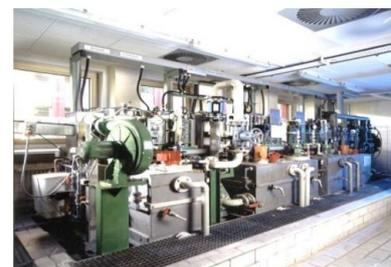
Figure 11. Electro galvanising pilot line (TKSE).
