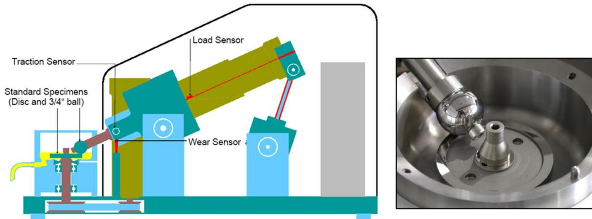
Figure 2. Mini traction machine (performance of the emulsion in the Roll Bite Mimicking Test, RMBT) (QH).
