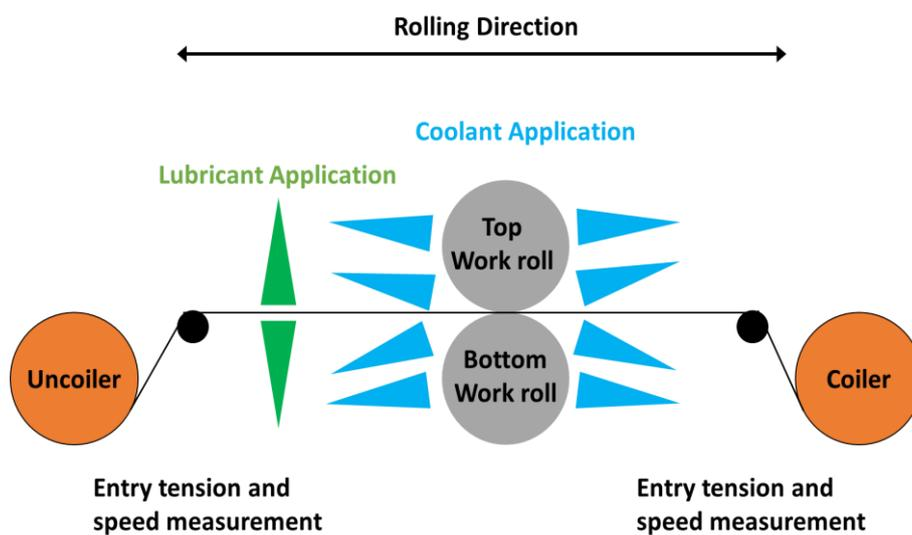
Figure 6. Scheme of the pilot plant of Tata.
