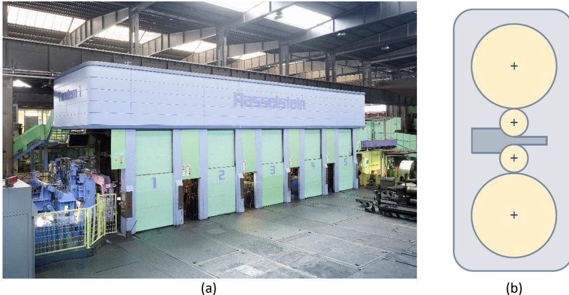
Figure 8. a) 5 stand tandem mill at TKPS; b) setup of a quarto stand of a tandem rolling mill, consisting of two back-up rolls and two work rolls.
