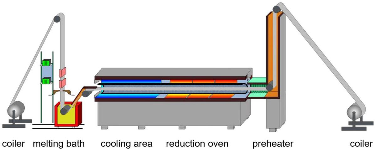
Figure 10. Hot dip coating pilot line (TKSE).
