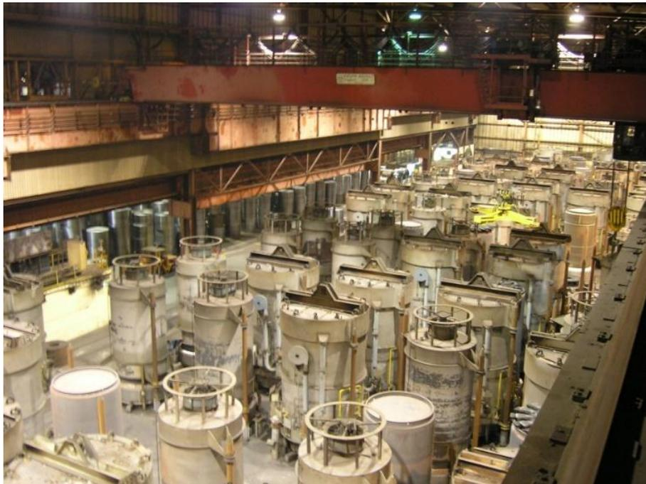
Figure 9. Batch annealing at TKSE Bochum.
