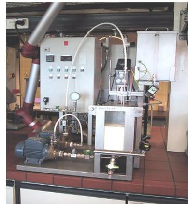
Figure 3. Lubricant recirculation test.
