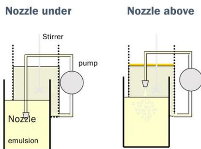
**Variables:** Retention time (volume/nozzle), Pressure, Temperature, Concentration, Water type, with/without air impact, Agitation (stirrer).
